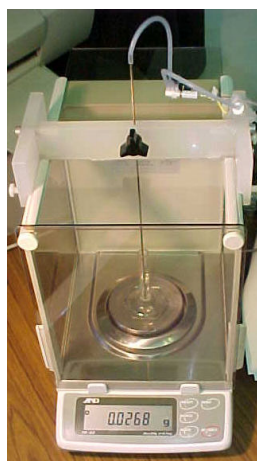
Fig. 8. Microscale system used to measure very low liquid mass flow rates.
